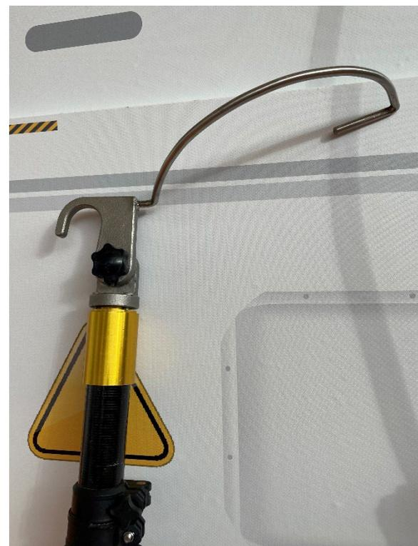
**Step.2 Extend the pole.** Unlock the locking on the top extendable section, extend and fasten the lock again after full extension and then open the second extendable section and repeat again for the rest of the sections until reaching the desired height.
