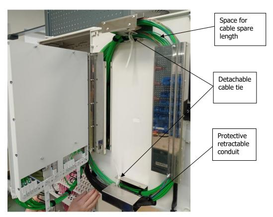
Fig.7. Disassembled inner box.
