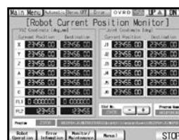
Current position monitor screen
