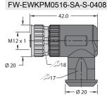
Field-wireable female connector, M12 × 1, angled, 5-pin, screw terminal connection, cable feedthrough 4.0 to 8.0 mm, core cross-section/terminal capacity 0.25 to 1.5 mm², plastic housing, metal nut
