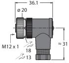
Field-wireable female connector, M12 × 1, angled, 5-pin, screw terminal connection, cable feedthrough 4.0 to 6.0 mm, core cross-section/terminal capacity 0.25 to 0.75 mm², plastic housing, metal nut
