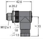
Field-wireable connector, M12 × 1, angled, 4-pin, screw terminal connection, cable feedthrough 4.0 to 6.0 mm, core cross-section/terminal capacity 0.14 to 0.75 mm², plastic housing, metal retaining screw
