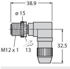
Field-wireable male connector, M12 × 1, angled, 4-pin, insulation piercing connection, cable feedthrough 4.0 to 5.1 mm, core cross-section/terminal capacity 0.14 to 0.34 mm², plastic housing, metal nut
