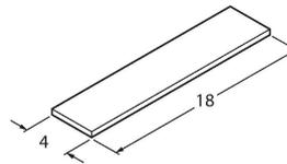
Label for TEL and TXL cables, length: 18 mm, height: 4 mm, material: polycarbonate (PC), color: white, halogen-free and flame-retardant
