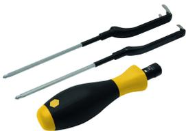
Torque wrench set; handles with adjustable torque 0.4-1.0 Nm, torque wrench for M8 (SW9), fork wrench for M12 (SW 14)
