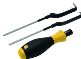
Torque wrench set; handles with adjustable torque 0.4-1.0 Nm, torque wrench for M8 (SW9), fork wrench for M12 (SW 14)
